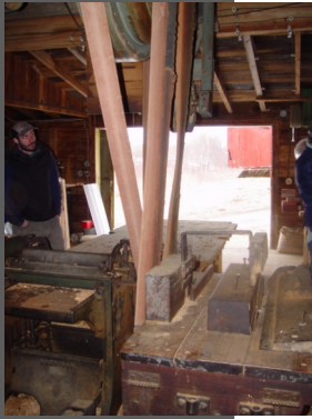
Belts powered by water once ran a table saw inside Masse Mill.
